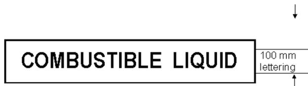
*Figure 5—Placard for C1 combustible liquids*
