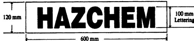
Figure 1—Form and dimensions of an outer warning placard
